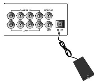
Connect one DC 12V, 6.6 A Adaptor to the back side of Power Jack.
